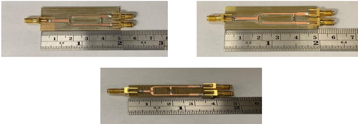
Figure 43: Photographs of the Milled Wilkinson Power Dividers with (a) Step Junction, (b) Taper Junction and (c) Straight Dividers.
